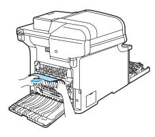
6 Close the fuser cover (1) and lift the two green levers at the left and right hand sides.
